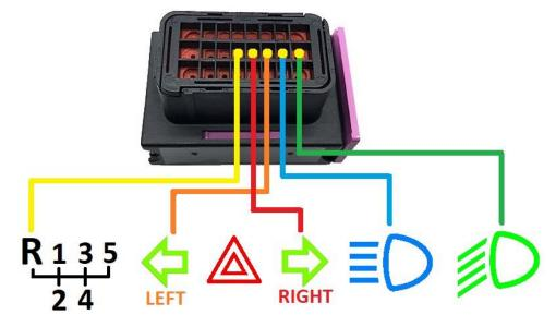
Pin B1: Input 4 (Low Beam lights +12V)
